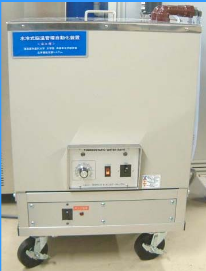
Reservoir for warm water
